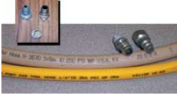
Figure 1. Large vs. small capacity quick-disconnects (above) and 1/4-inch vs. 3/8-inch air hose diameters.
